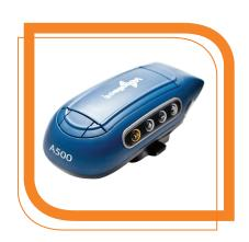
The Vocollect Talkman® A500 is an extensible voice-centric mobile computing voice appliance that enables high-performance, hands-free, and eyes-free workflows. It is the first Vocollect device to leverage the Next-Generation Vocollect Voice® software suite based on VoiceCatalyst®, making it the best solution to enable voice in all of your workflows throughout your distribution centre (DC) or warehouse.
